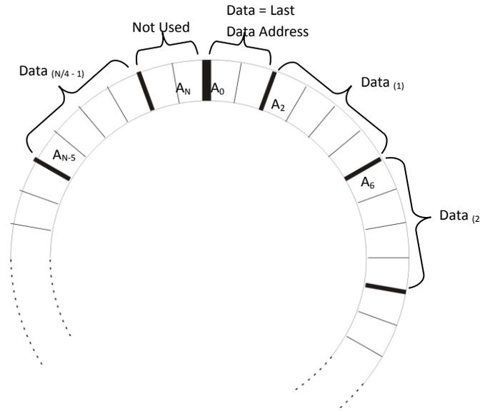
Fig. 4 Temperature data arrangement in the EEPROM memory
