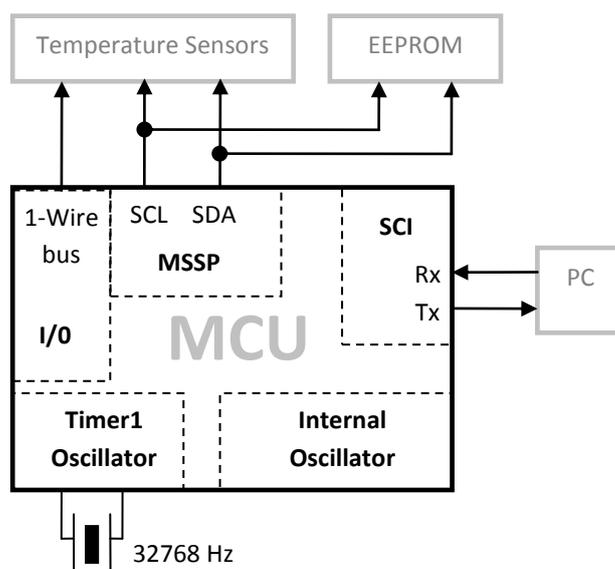
Fig. 3 Block diagram of the embedded system
