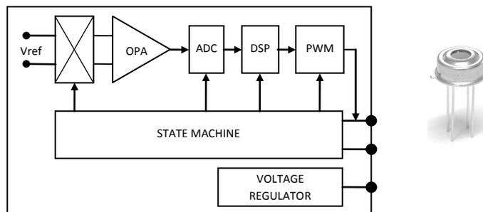
Fig. 2 Simplified block diagram of MLX90614 temperature sensor
