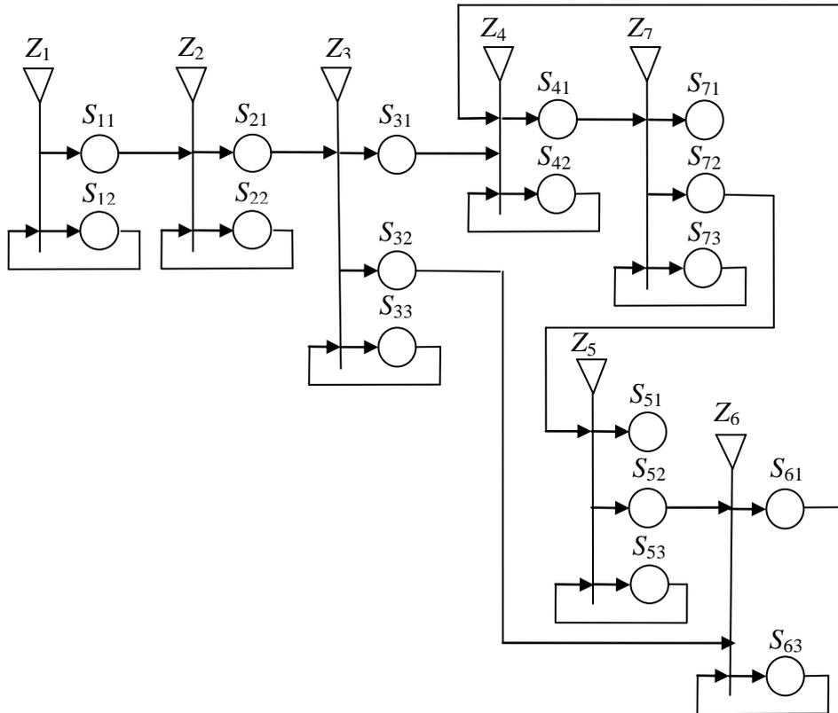
Fig. 5 GN model of the temperature data logger system
