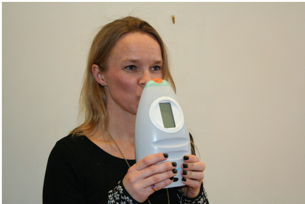
Fig. 2. Measurement of nitrogen oxide in exhaled air (NIOX MINO). Photo: Robert Wålinder
