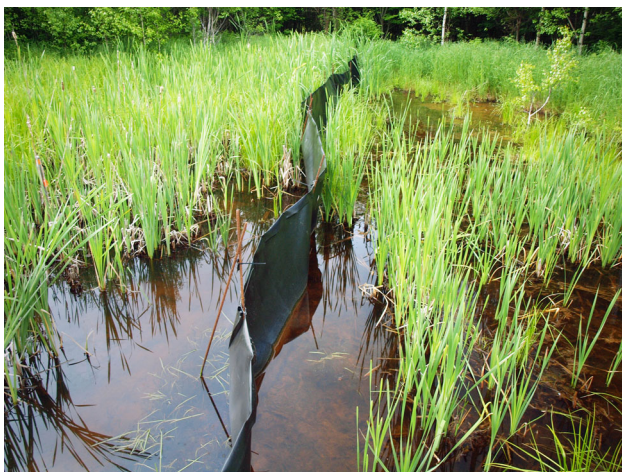
Fig. 1 HDPE barrier dividing an experimental wetland
