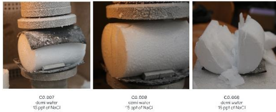
Figure 8. Ice specimen with 15ppt of NaCl, before, during and after the compression test at -70^{\circ}\text{C} .
