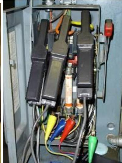
**Figure 3: Power Measuring Device Connected to Fadal CNC Machine**
