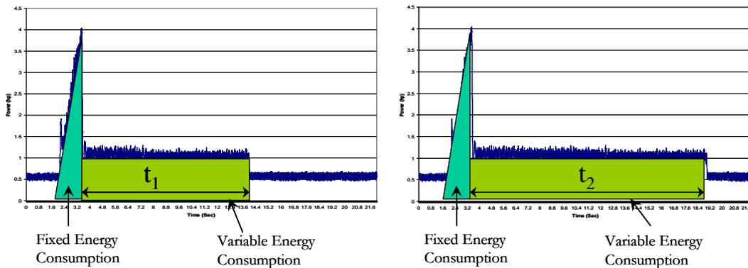
**Figure 1: Fixed Energy Consumption vs. Variable Energy Consumption**
