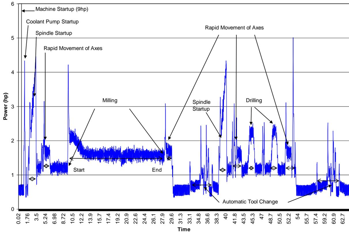
**Figure 4: Power Plot for CNC Mill**
