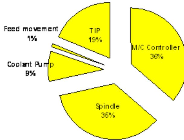
**Figure 6: Energy Distribution for Milling Process**
