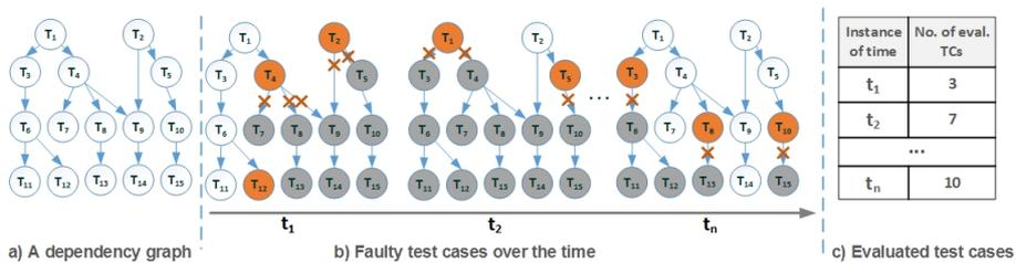
**Figure 3.** A dependency graph. (a) A dependency graph showing 15 test cases (TCs) with arrows indicating dependencies; (b) faulty test cases (orange) over time after each ontology modification; and (c) number of evaluated test cases (TCs) per instance of time. Every instance of time, the set of test cases is completely evaluated.
