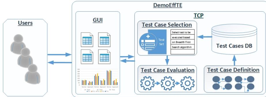
**Figure 1.** The architecture of the DemoEffTE demonstrator. Users are able to choose different scenarios for evaluation of the EffTE approach compared to a naive approach, as well as a set of test cases and their dependencies; the result of the validation process is returned as output.
