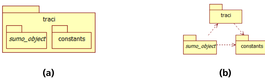
Figure 12-2: The TraCI-Python API components: (a) deployment, (b) Dependency relationships.
