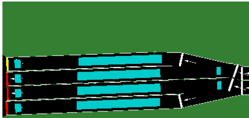
Figure 3-2: Typical detection field for vehicle actuated control
