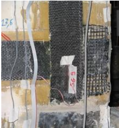
Figure 8. Anchorage at the free extremities
