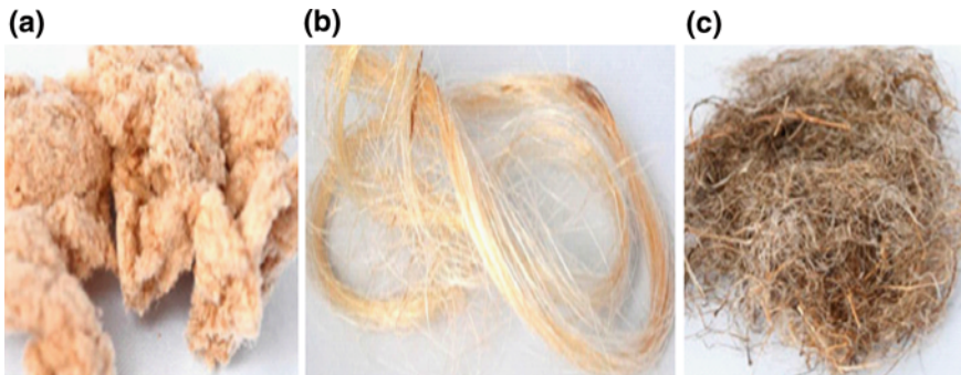
Fig. 1 Vegetable fibres as a pulp, b strands and c staple [25]
