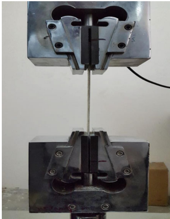
Fig. 4 Tensile test setup with the composite specimen loaded on to the UTM
