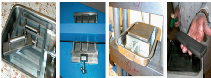
Fig. 3 Mould and press system to prepare the specimens [25]
