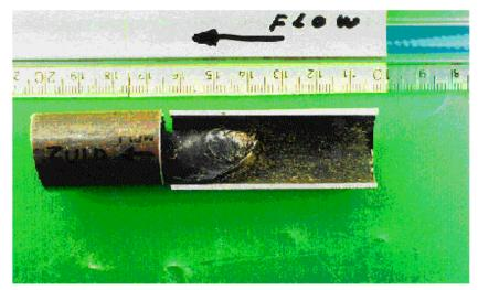
> 2: Clamping musselshells were observed inside the tube. Hole is localised under the musselshells.
