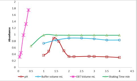
**Figure 4-** Effect of pH, buffer volume, EBT (0.01%) volume, and shaking time on absorbance of the orphenadrine –EBT ion-pair.
