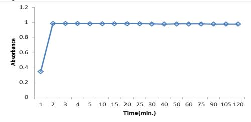
Figure 5- Effect of the time on the stability of ion pair complex.
