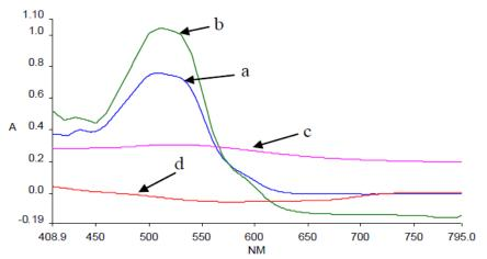
**Figure 3-** Absorption spectrum of a- 3  $\mu$ g/mL orphenadrine citrate- EBT ion pair complex b- mixture of paracetamol and orphenadrine citrate -EBT ion pair complex (4.5  $\mu$ g/mL orphenadrine and 40  $\mu$ g/mL paracetamol) c- paracetamol aqueous layer, and d- paracetamol organic chloroform layer.
