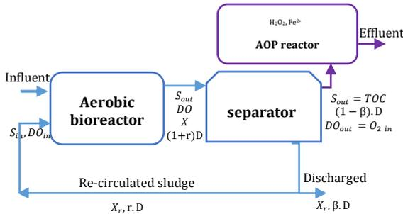
Figure 1: Block diagram of the integrated process.
