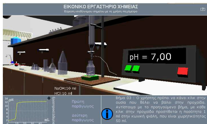
Fig. 4. The pH is presented on the screen of the pH-meter. The process completes when the pH value remains almost constant at the equivalent point
