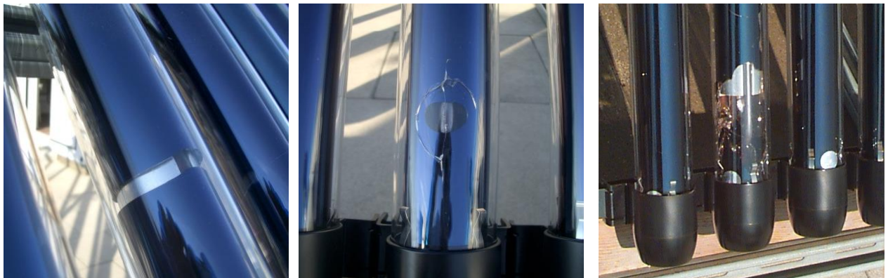
Figure 2: Damaged collectors after testing; Fraunhofer ISE
