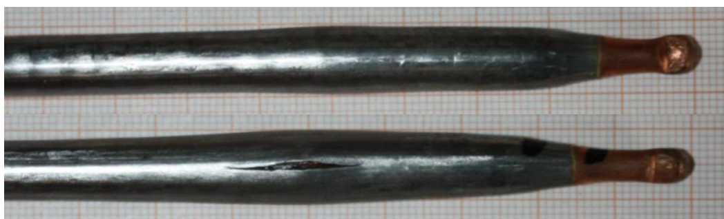
Figure 3: Heat pipes after freeze resistance test (Source: HPQUAL - Investigation of freeze resistance testing of heat pipes; Fraunhofer ISE)
