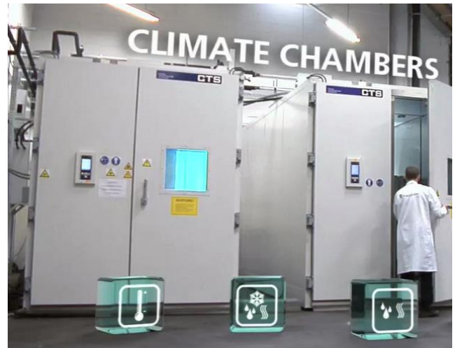
Figure 1: Climate chambers of the TestLab PV-Modules, Fraunhofer ISE
