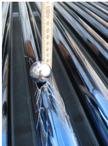
Figure 3: Damaged collector after steel ball impact test
