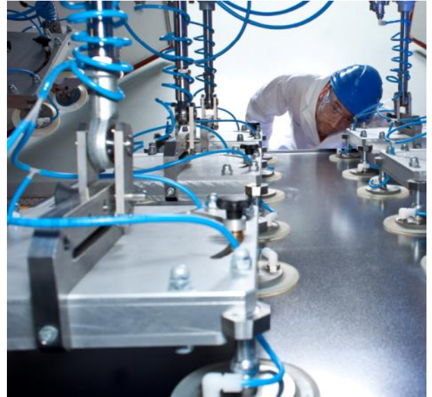
Figure 1: Mechanical load test; Fraunhofer ISE
