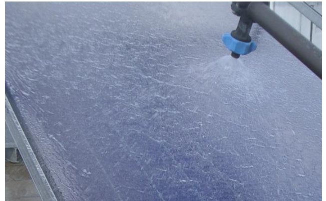
Figure 1: External Thermal Shock Test; Fraunhofer ISE
