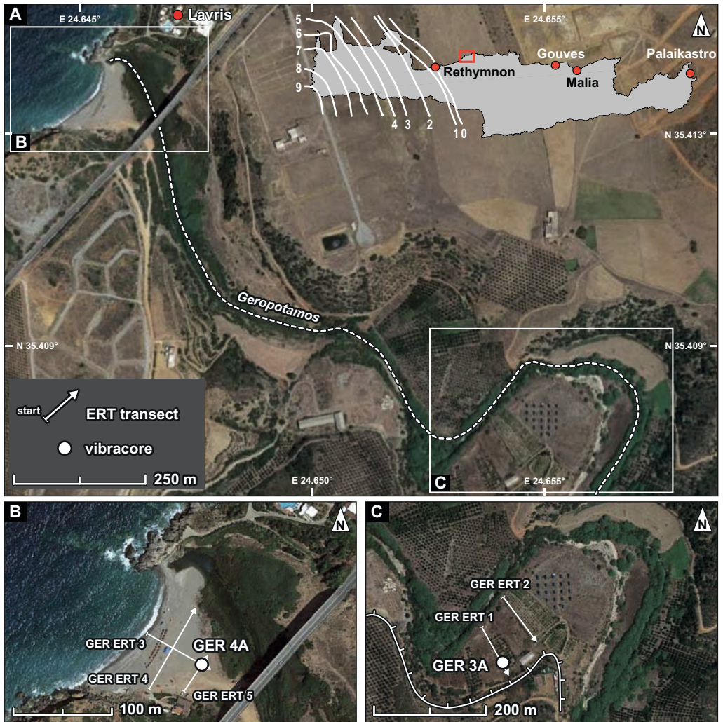
Fig. 1. Overview of the lower course of the Geropotamos River and the river mouth area into the Cretan Sea (A). Detail maps of the Geropotamos River mouth area (B) and the inactive external bank further inland (C) show locations of vibracoring sites and ERT transects. Isolines in inset map of Crete depict amount of coseismic uplift associated with AD 365 earthquake in meters (after Kellat 1991, Shaw et al. 2008). Maps based on Google Earth 2017.
