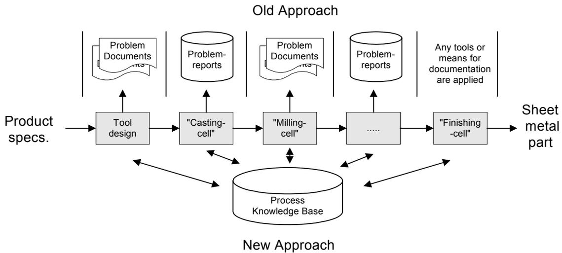
Figure 3: Management of knowledge in a process chain for formed sheet metal parts
