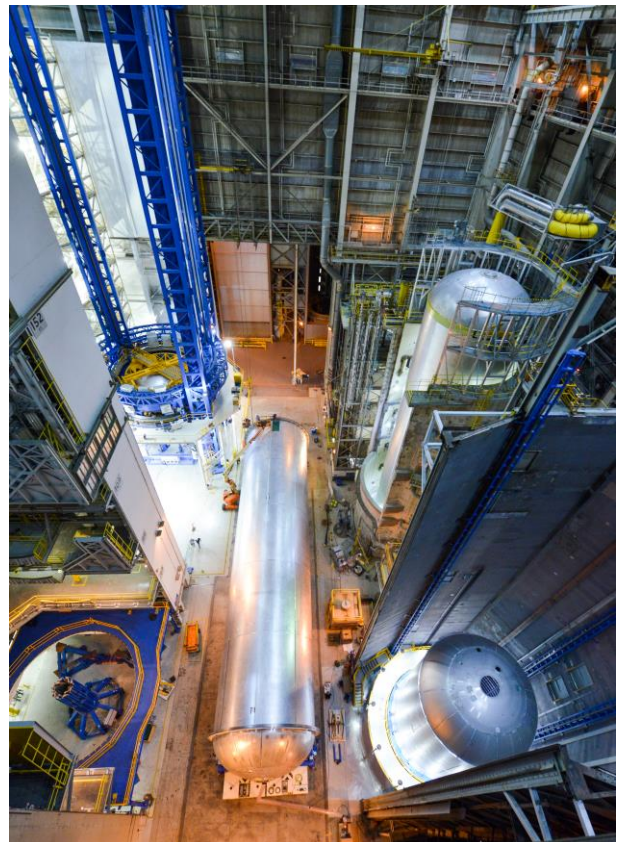
Figure 3. SLS propellant tanks manufactured at Michoud Assembly Facility
