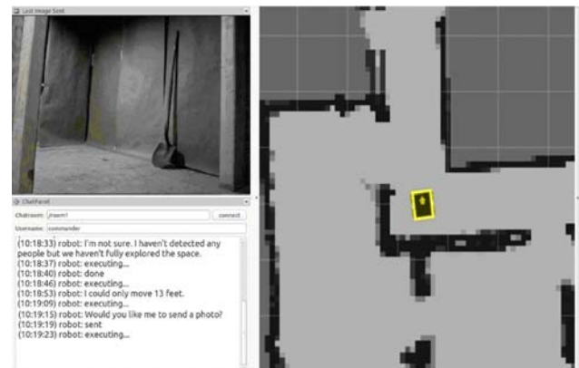
Figure 1. Visual and language components of robot-to-human interface: robot text responses (lower left), LIDAR-generated map (right), last still image requested from robot (upper left). The human-to-robot interface was a microphone for spoken natural language.
