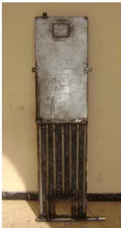
Fig. 2 Absorber made by tubes and galvanized tank
