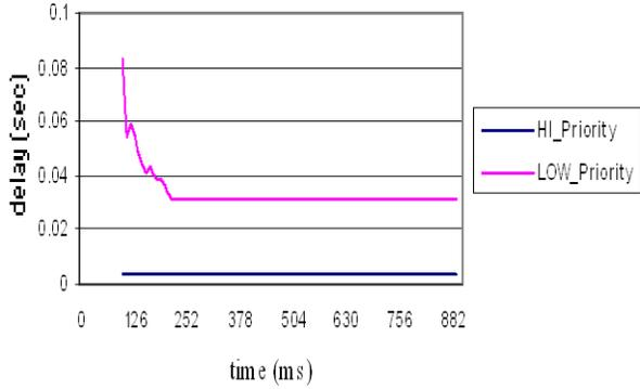
Fig. 5. End-to-End Delay with Different ToS
