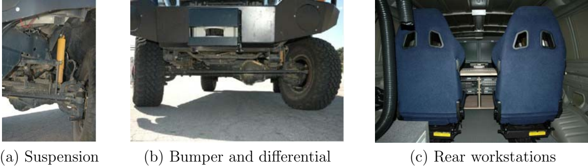
Figure 2: Offroad modifications by Sportsmobile, Aluminess and Team Caltech.
