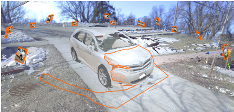
Fig. 1 An example image showing a 3D capture of an automobile, including sampling locations (orange outlined photographs)
