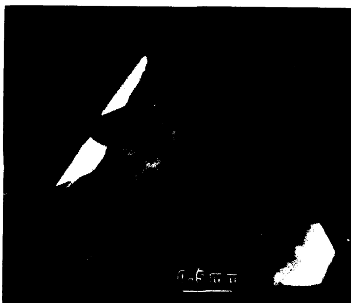
Figure 1. Optical micrograph of an as-grown crystal of Py-D3C exhibiting a characteristic truncated octahedral shape. Domains are apparent in transmitted cross-polarized light.
