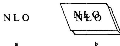
Figure 11. (a) An image (b) appears to be doubled when viewed through a birefringent material.
