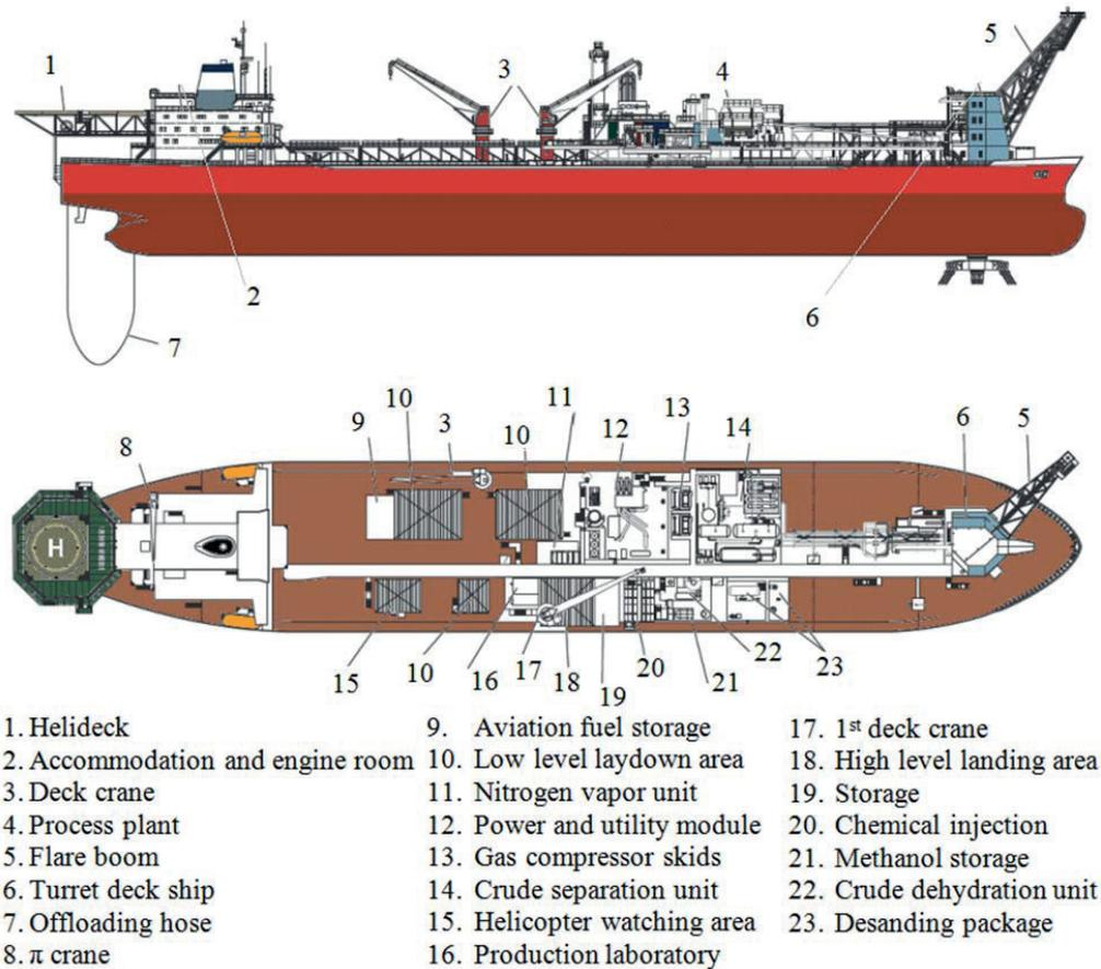
Figure 1. The typical FPSO module layout (“Floating production system,” 2009)
