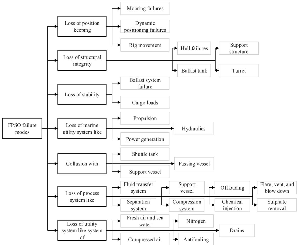
Figure 2. The common failure modes of FPSO system (Bhardwaj *et al.*, 2017)
