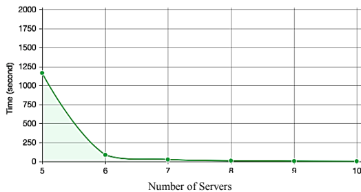
Fig.4. Relationship between no. of agents and average waiting time in Erlang C model
