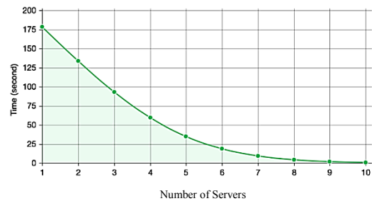
Fig.6. Relationship between no. of agents and average waiting time in Erlang A model
