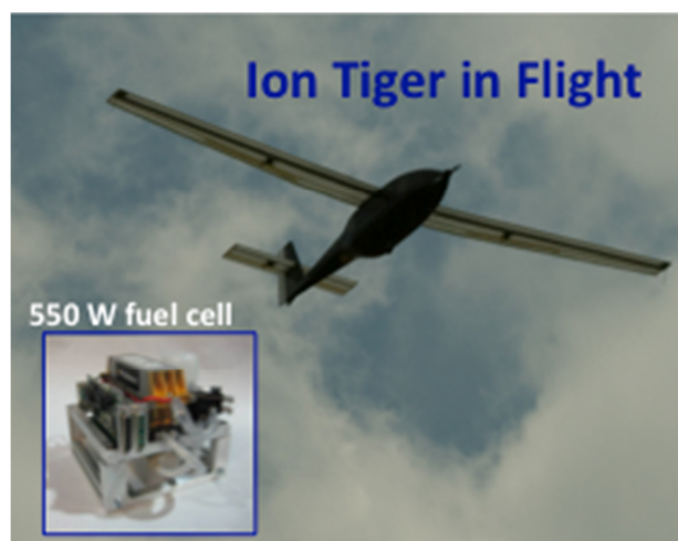
Figure 1. Ion Tiger UAV in flight. The Ion Tiger gross takeoff weight (GTOW) is 16 kg, with 40% of its weight budget allocated to the propulsion/energy system. The wingspan is 5.2 m, with a lift over drag ratio near 17 (2). The inset shows the Ion Tiger's 1.1 kg ~550W fuel cell system built by Protonex Technology Corporation.
