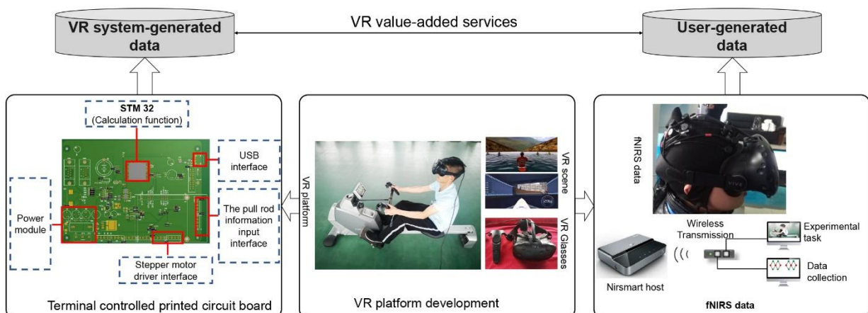
Figure 2. The system architecture of the smart VR rowing machine.
