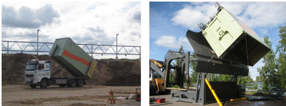
FIG. 2. Back-dumping of biomass containers (left) and unloading of containers with an open roof by the dumping system (right).
