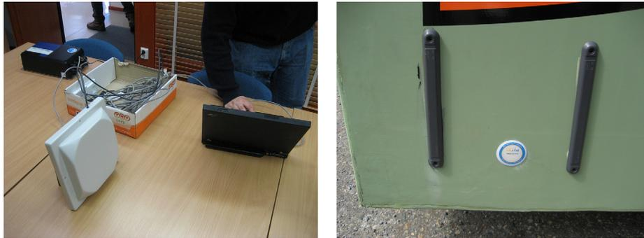
FIG. 1. Reading hardware for a reader gate and RFID tags, oblong for reader gate and circular for smartphone.
