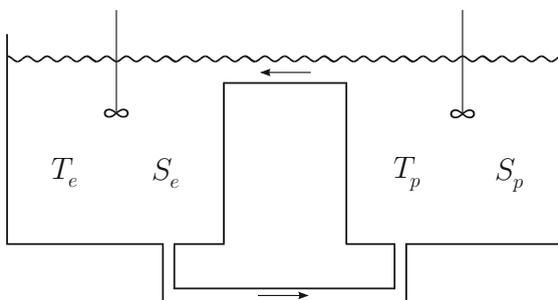
**Fig. 1** Diagram of the two-box Stommel model, based on [14, Fig. 5]:  $(T_e, S_e)$  represent equatorial temperature and salinity, respectively, and  $(T_p, S_p)$  represent polar temperature and salinity. The boxes are connected on top by an overflow and on the bottom by a capillary tube. The flow rate between the two boxes is assumed to be equal and of opposite signs through the overflow and capillary tube
