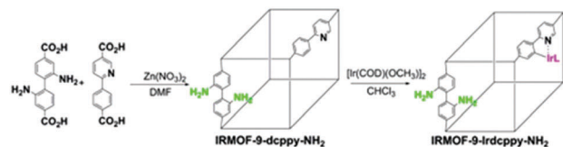
Scheme 7 Synthesis of IRMOF-9-Irdcppy-NH 2 by PSM. Reproduced from ref. 39 with permission from American Chemical Society.
