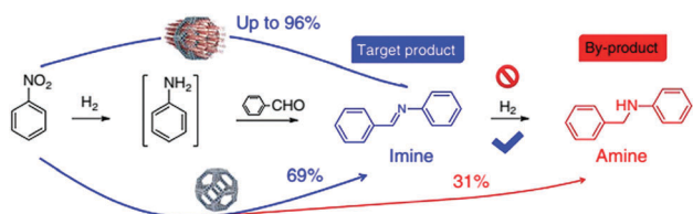
Scheme 26 Size-selective catalysis of nitrobenzene reductive imination. Reproduced from ref. 145 with permission from Nature Publishing Group.
