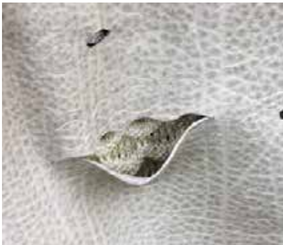
Fig. 5. The cuts realized by laser technology to connect the internal and the external part
