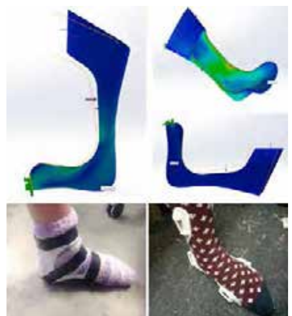
Figure 3. Early printed orthosis and strength analysis
