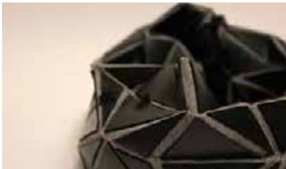
Fig. 1. Surface detail of the demonstrator: rubber with cotton fabric. (© Ruben Daems)
