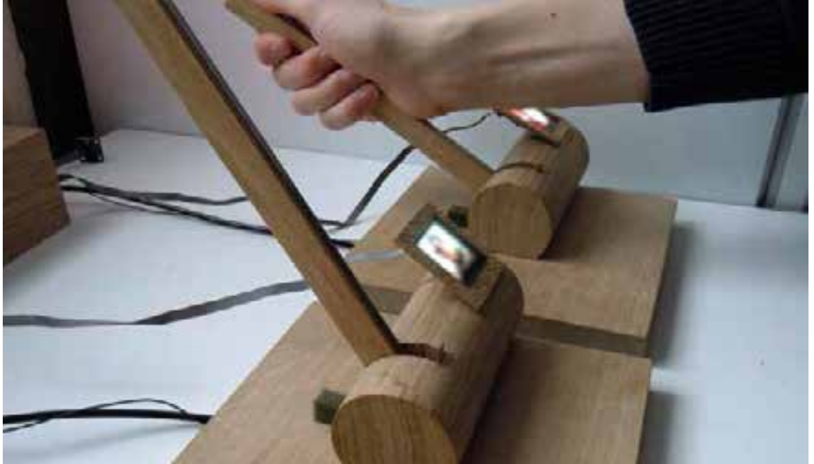
Fig. 2. The Physical Meeting Manager used to arrange a meeting by pressing down the lever. Haptic feedback of the lever conveys the intentions of the other side.
