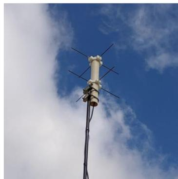
**Figure 5. Turnstile Antenna Design**
