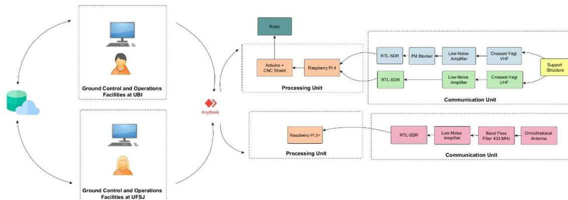
Figure 6. Ground Segment Overall Architecture
