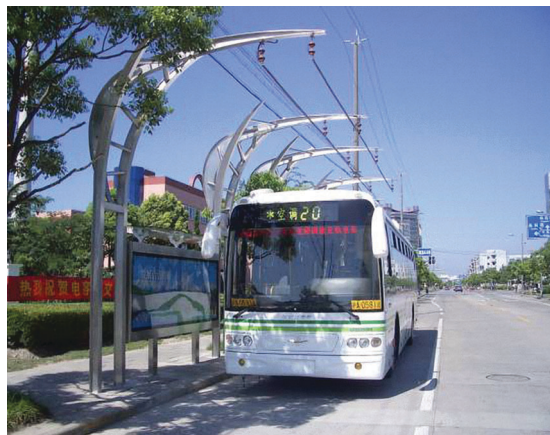
Fig. 16 Trolley bus of Aowei Technology Co., Ltd, based on Ni(OH) 2 /AC supercapacitor. 177
