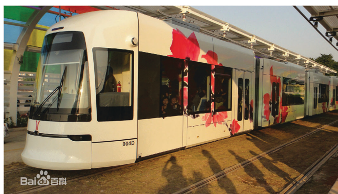
Fig. 17 Electric tramcar of CSR Co., Ltd, based on AC/AC supercapacitor. 178
