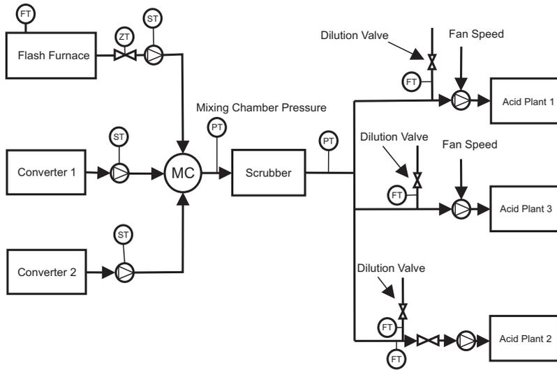
Figure 5: Process, manipulated variables and disturbances
