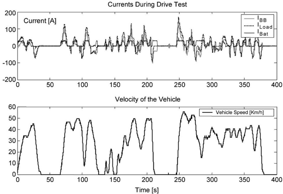
Fig. 4. Driving test fragment of currents and speed.
