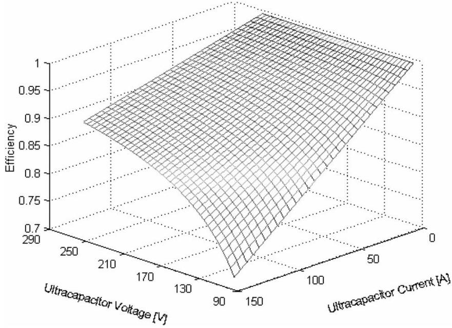
Fig. 5. Efficiency map of the boost converter.
