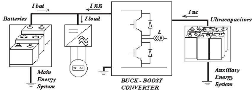
Fig. 2. Resulting power circuit in the EV.
