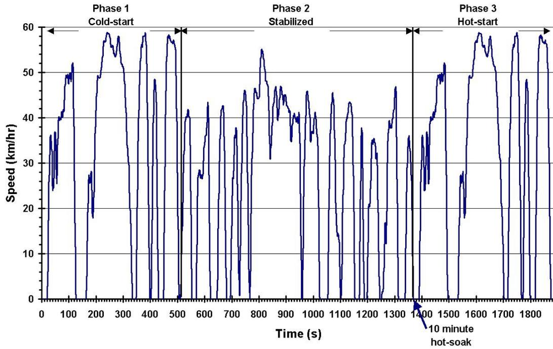
Appendix Figure 1: Class 1 (<170 cc) Motorcycle FTP Urban Dynamometer Drive Cycle
