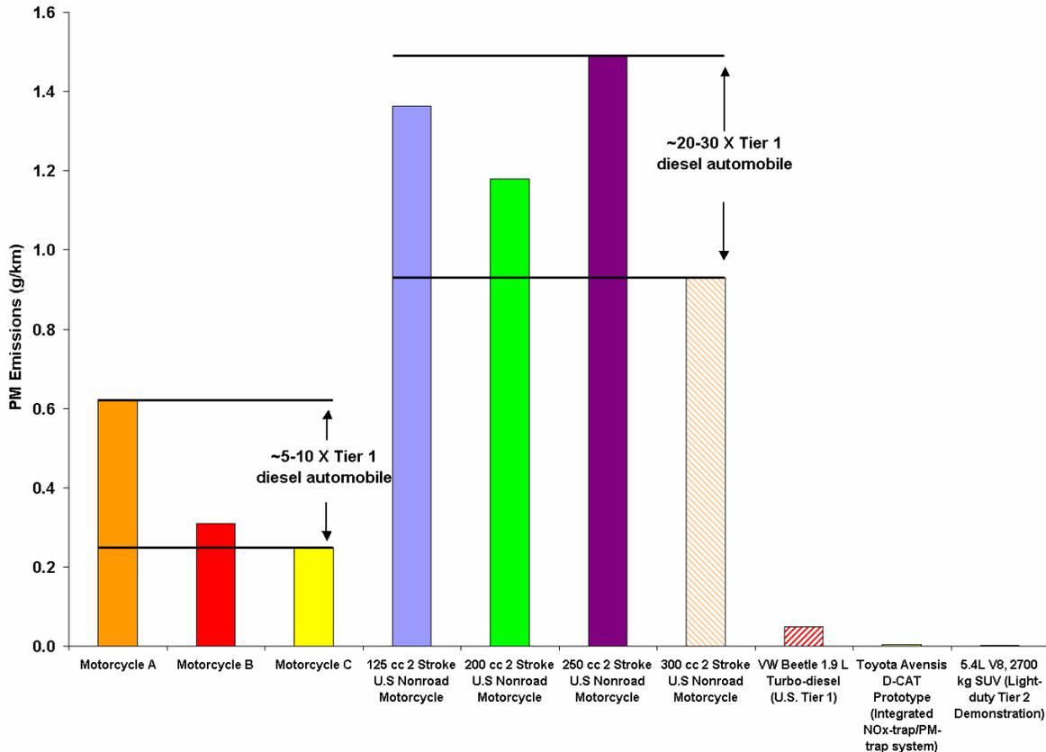
**Figure 4:** A comparison of PM emissions from the tested motorcycles to that of other motorcycles and light-duty vehicles tested at the U.S. EPA – NVFEL.
