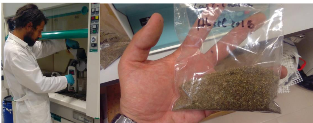
Figure 1. Images of the aerial biomass mill process (left) and final milled biomass (right)
