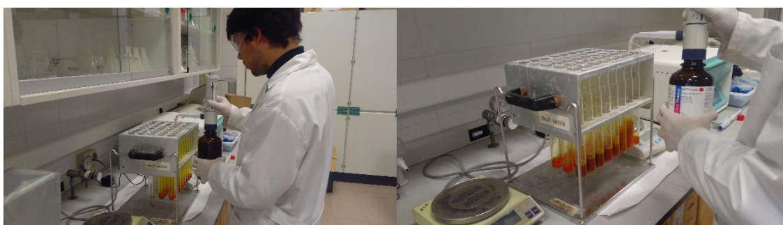
Figure 4. Images of the potassium dichromate (left) and sulphuric acid (right) addition.
