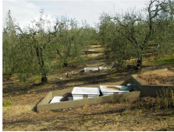
Figure 3. Picture showing the tree-tanks systems installed in each of the plots to collect the water and sediment (Photograph of Instituto de Agricultura Sostenible, CSIC). Experimental design, collectors set up and sampling were performed by Instituto de Agricultura Sostenible, CSIC under the supervision of J. A. Gómez Calero) ( Instituto de Agricultura Sostenible, CSIC ).
