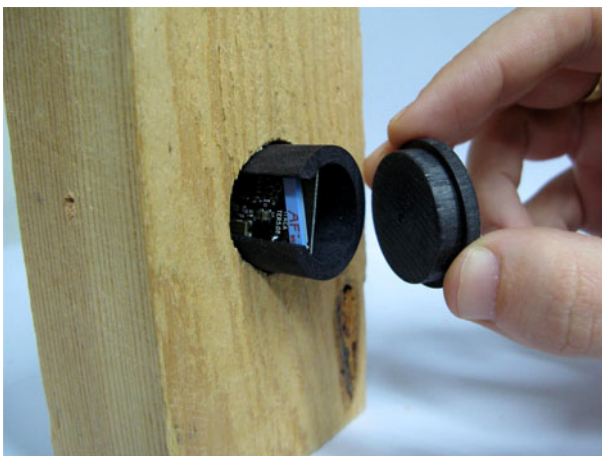
Fig. 8 Insertion of the sensor in the wood. The sensor is inside an open black-painted wooden housing to allow light reflection and entrance of termite workers
