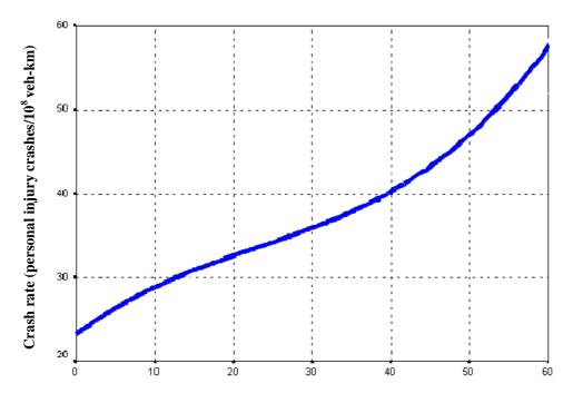
Design speed reduction from adjacent segments (km/h)
