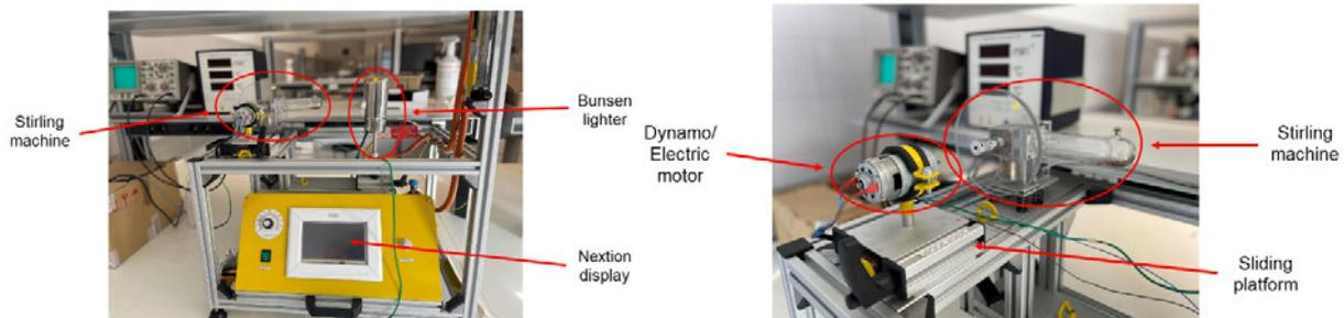
Figure 6. Test bench in its final state.
