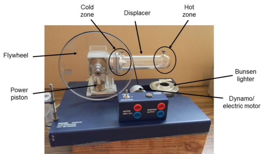
Figure 1. Initial state of the laboratory Stirling Machine.
