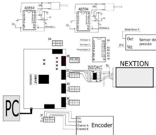
Figure 3. Connection of the final electronic circuit.
