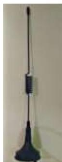
**Figure 11 118MHZ Antenna**
