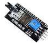
**Figure 6 I2C Converter**
