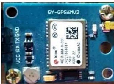
**Figure 9 Neo6M GPS module**
