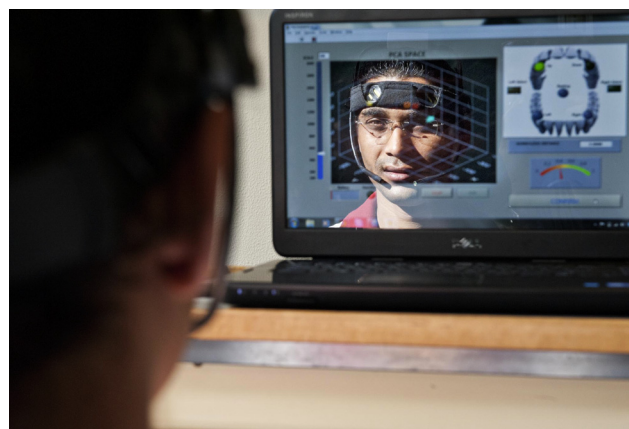
Fig 1 Participant wearing headgear of the TDS with control of the computer cursor through the magnet attached to the tongue. (Illustration courtesy of Ole Hein Pedersen.)
