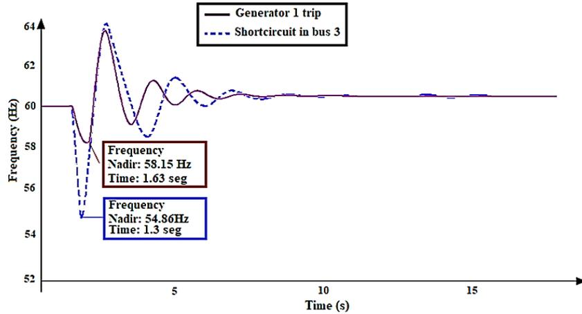
Figure 6. Frequency behavior in short circuit and generation loss events
