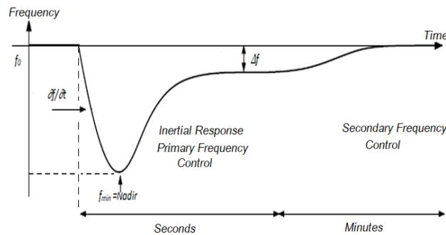
Figure 1. Frequency behavior stages in generation loss event
