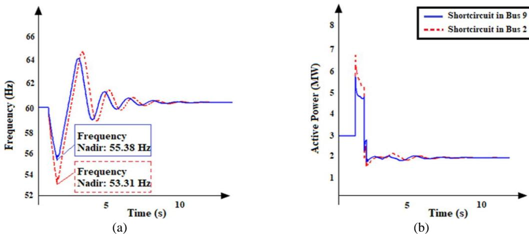
Figure 7. Short-circuit analysis (a) frequency behavior over time and (b) electric power delivered
