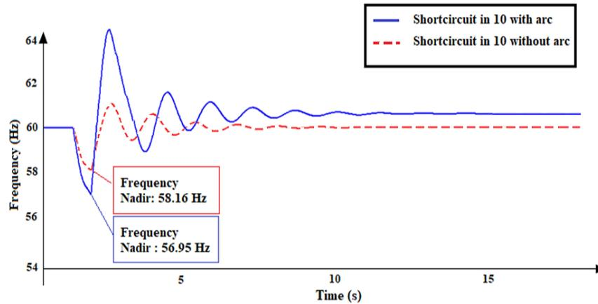
Figure 9. Behavior of the frequency under faults with the presence of the arc
