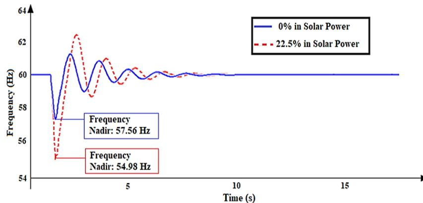
Figure 10. Frequency behavior in the event of a two-phase short circuit to ground in 75% of the line that interconnects nodes 9 and 10 for different penetration level of photovoltaic solar energy
