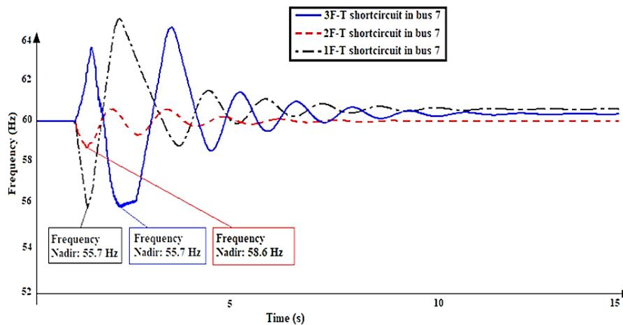
Figure 8. Frequency behavior for different types of short circuits
