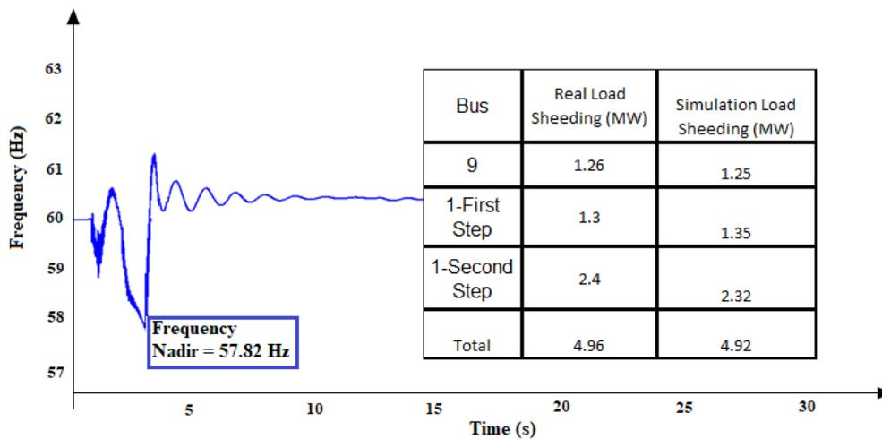
Figure 5. Frequency vs time in failure simulation
