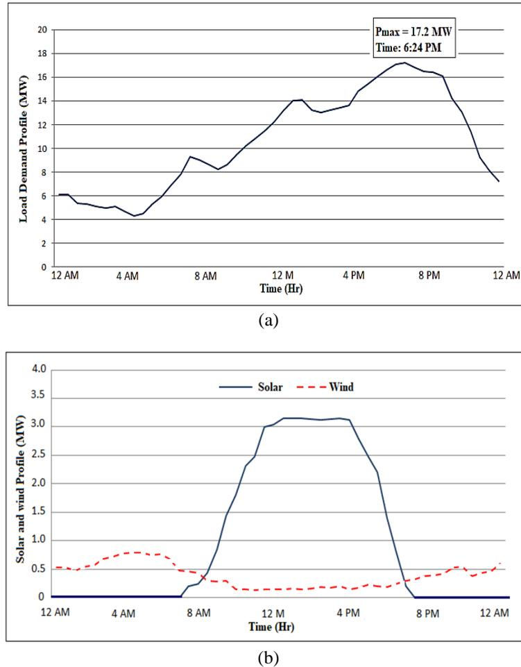
Figure 3. Demand and RESs generation profile where (a) demand daily behavior and (b) typical solar and wind generation in electrical system study case
