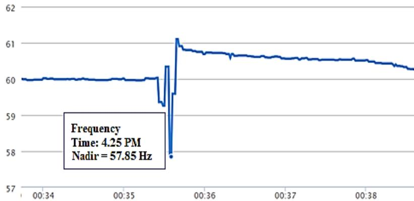
Figure 4. Actual frequency measured by frequency counter during failure studied
