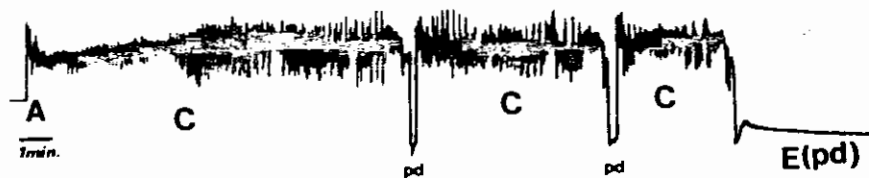
Figure 3.1. Electrical penetration graph (EPG) of Trialeurodes vaporariorum probing in a cucumber leaf (after Janssen, Tjallingii and van Lenteren, 1989). A whitefly is included in an electrical circuit via a gold wire attached to its thorax. Changes in electrical properties as a result of penetration activity lead to a characteristic pattern. During this penetration two short penetrations of cells occurred (pd), and, finally, a phloem sieve element was penetrated intracellularly (E(pd)). Pattern A reflects leaf surface penetration and pattern C represents intercellular penetration and salivary-sheath secretion. See Tjallingii (1988) for details about the methodology.
