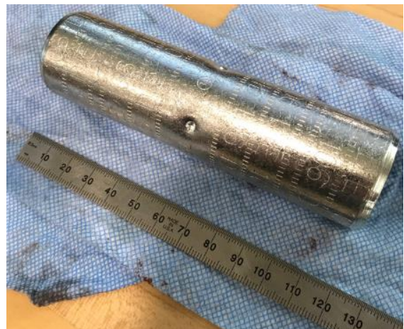
FIGURE 12: 750 MCM COPPER SPLICE BEFORE CRIMP.
