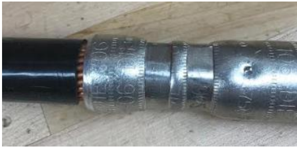
FIGURE 13: 750 MCM COPPER SPLICE AFTER TWO CRIMPS.
