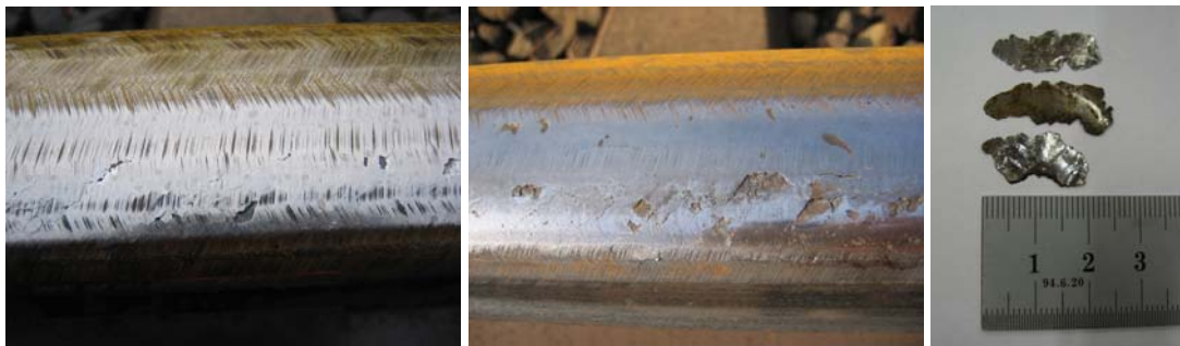
Figure 8: Surface fatigue cracks on high rail on the Malmbanan, 9 th September and 15 th September and worn-off flakes, (scale in millimetres).
