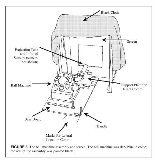
black cloth that was draped over the ball machine. The cloth prevented light from entering the enclosure. In addition, the ball machine was dark blue in color; thus, receivers were unable to tell in which direction the ball would be projected.
