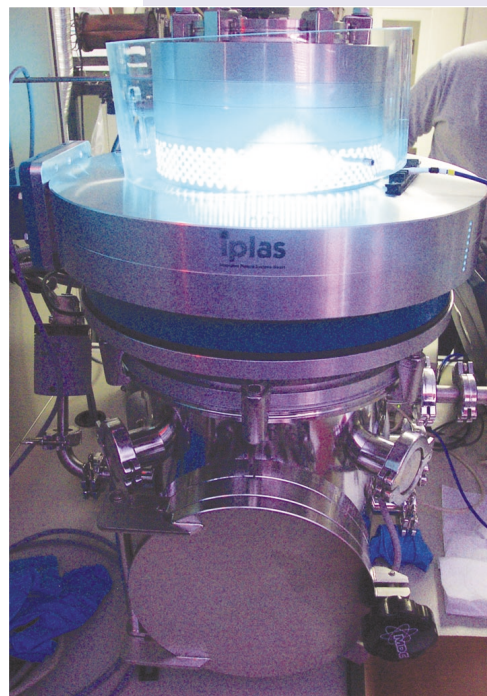
Fig. 3. Picture of the microwave plasma system used to grow UNCD thin films at Argonne National Laboratory. The emerald green color is derived from the C 2 dimers created in the plasma.
