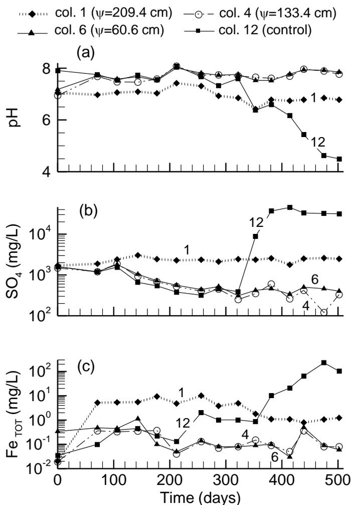
Figure 2. Observed drainage water evolution during leaching of the 4 columns, showing (a) pH, (b)  $\text{SO}_4^{2-}$  and (c) total Fe. Water suctions refer to the suction head applied at the base of the column. Each point corresponds to the beginning of a drainage cycle (effluent concentrations were measured within 1-2hrs. after adding water).
