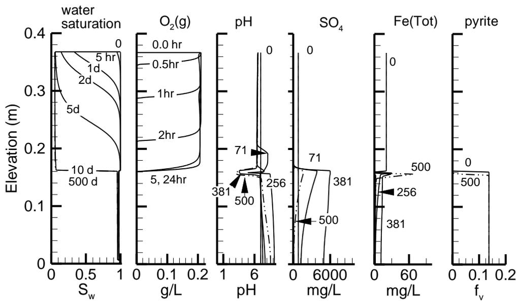
Figure 4. Simulated vertical profiles for column 6 (suction head = 60 cm) showing water saturation,  $O_2$ , pH,  $SO_4^{-2}$  and Fe concentrations, and pyrite volume fraction at selected times (times in days unless otherwise noted).
