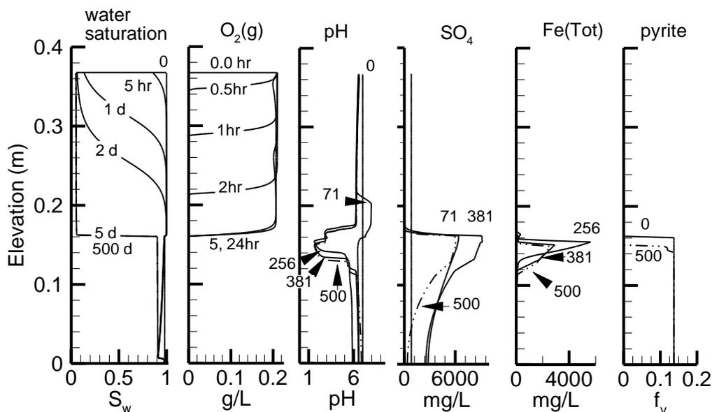
Figure 3. Simulated vertical profiles for column 1 (suction = 209 cm) showing water saturation,  $\text{O}_2$ , pH,  $\text{SO}_4^{-2}$  and Fe concentrations, and pyrite volume fraction at selected times (times in days unless otherwise noted).
