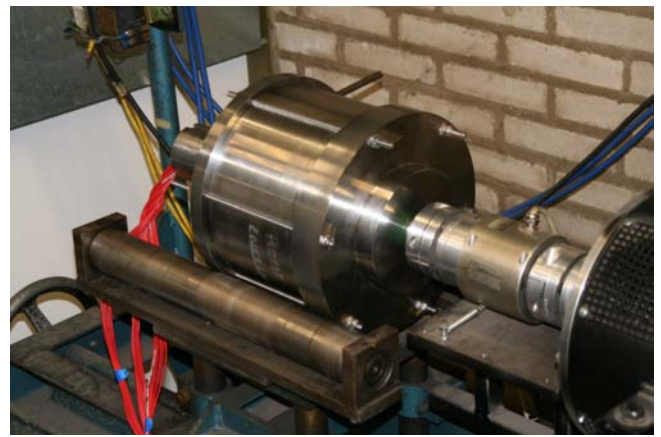
Fig. 9. Prototype direct-drive external rotor brushless permanent magnet generator on the test bench for initial measurements.
