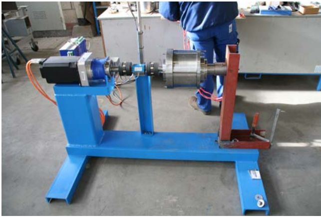
Fig. 10. Direct-drive external rotor brushless permanent magnet generator attached to a servo machine for power measurements.
