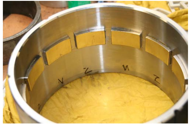
Fig. 6. External permanent magnet rotor with one of two rows magnets glued to the mildsteel back-iron.
